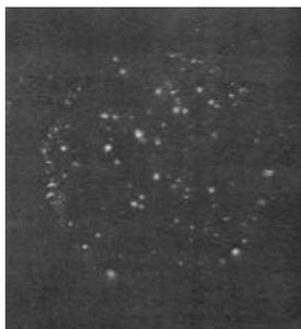
Fig. 13. Autoradiograph of Deuterated Ti Disc
