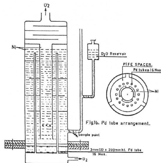
Fig. 1. Schematic View of Milton-Roy Commercial Electrolyzer
