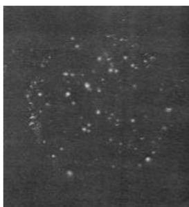
Fig. 13. Autoradiograph of Deuterated Ti Disc
